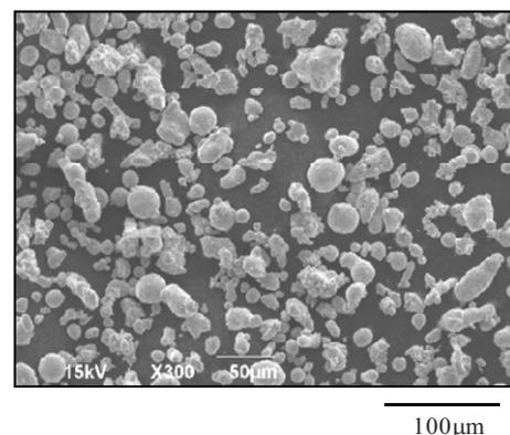
Fig. 1 SEM image of metal powder
