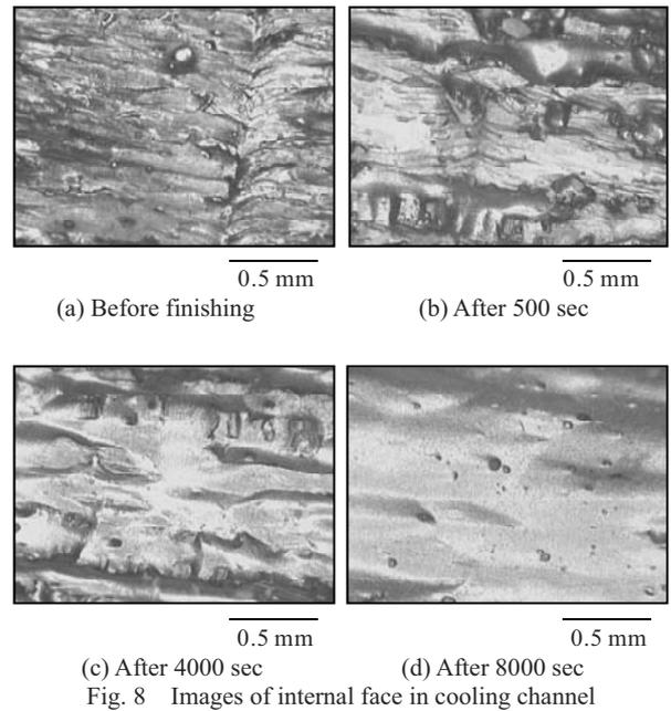
Fig. 8 Images of internal face in cooling channel
