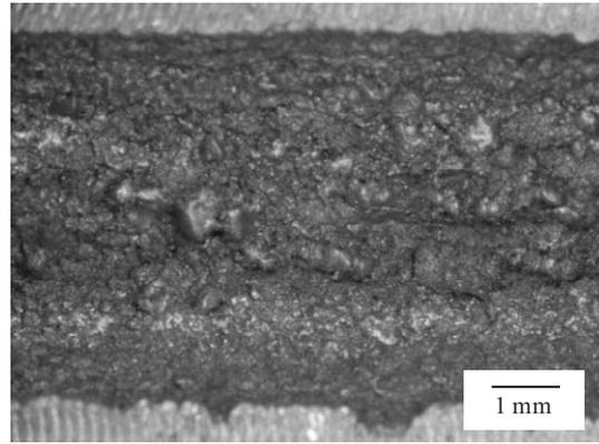
(a) Without face protuberance ( $R_z=109\ \mu\text{m}$ )
