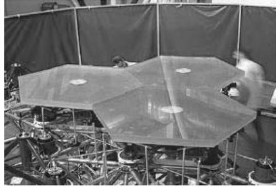
Fig. 4: Grantecan mirror segments being readied for optical testing using the REOSC test tower [16]
