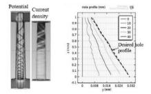
Fig.5 Simulation results with designed electrode (a) Potential and current density distribution at Time=40s, (b) Hole profile at Time=0s, 10s, 20s, 30s and 40s
