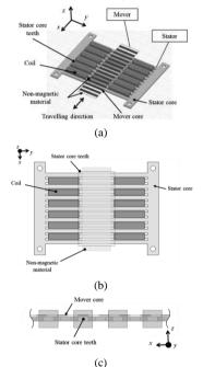
Fig.2 Basic structure of the LSRM (a) 3-D view (b) Top view of stator (c) Cross- sectional view
