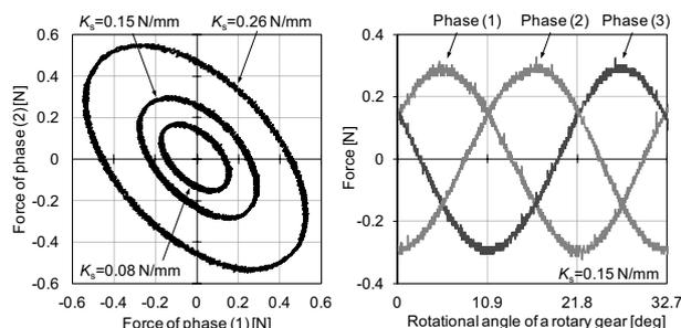
Fig. 4. Balanced tensional forces in SMA wires and springs when the rotor gear is rotated by an external force
