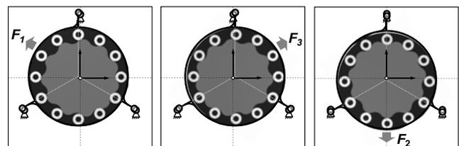
Fig. 2. Operating schematics of the rotational driving mechanism
