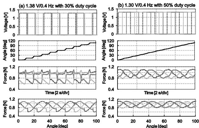
Fig. 5. Measured tensional forces and rotational displacement with different amplitudes of applied voltage and pulse duty cycles
