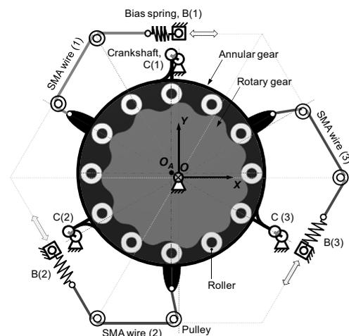
Fig. 1. Configuration of the bidirectional rotary actuator which consists of a rotational driving mechanism and three SMA wires with bias springs
