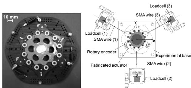
Fig. 3. A fabricated functional prototype of 160×150×25 mm with three SMA wires of 0.1 mm diameter and 50 mm length (left) and planar schematics of experimental setup (right)
