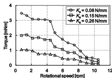
Fig. 6. Pull out torque vs. speed for different stiffness of the bias springs
