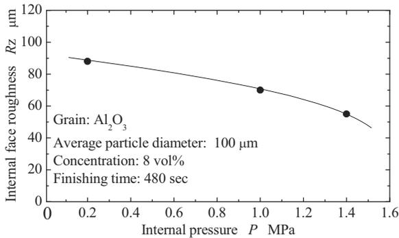
Fig. 10 Influence of internal pressure on finishing performance
