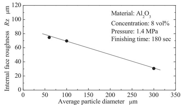
Fig. 9 Influence of grain size on internal face roughness
