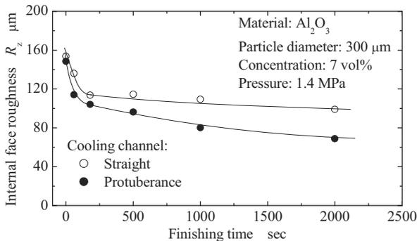
Fig. 11 Influence of face protuberance on internal finishing
