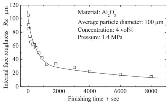
Fig. 7 Influence of finishing time on internal face roughness
