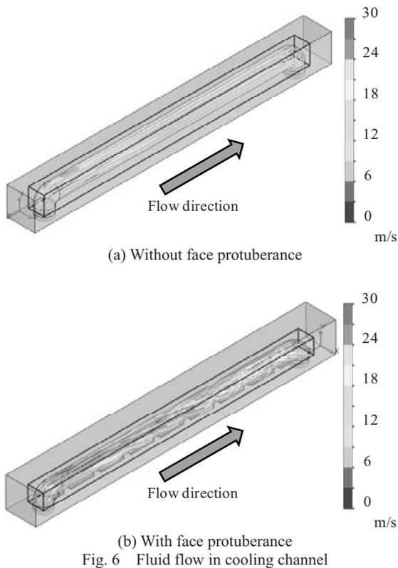
Fig. 6 Fluid flow in cooling channel
