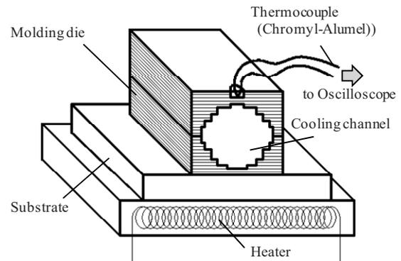
Fig. 5 Finishing equipment for internal face of cooling channel
