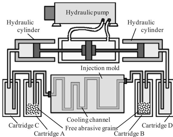
Fig. 2 Finishing equipment for internal face of cooling channel
