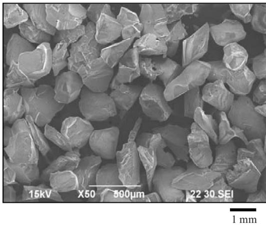
Fig. 4 SEM image of free abrasive grains (Material:  $Al_2O_3$ , Grain size: 100  $\mu m$ )
