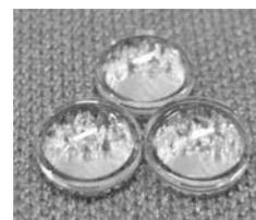
Fig. 8. Photograph of the molded aspherical lenses.
