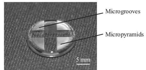
Fig. 13. Photograph of the molded microstructures on glass plate.
