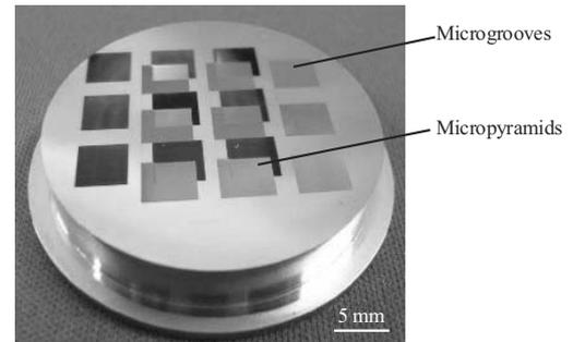
Fig. 12. Photograph of the mold for microstructures.
