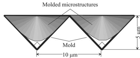
Fig. 11. Schematic diagram of the cross section of microgrooves and micropyramids.
