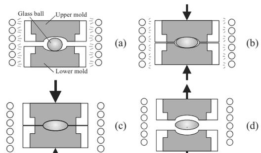
Fig. 1. Process flowchart of the IGMP process: (a) heating, (b) pressing, (c) annealing, (d) cooling.
