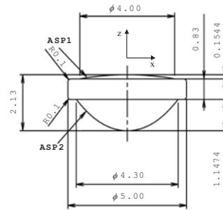
Fig. 4. Designed biconvex aspherical lens.
