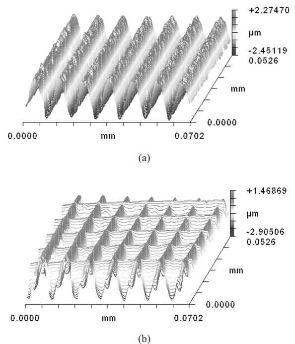
Fig. 14. 3D topographies of the molded microstructures on glass plate: (a) microgrooves and (b) micropyramids.
