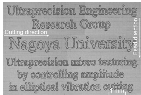
Fig. 16 Photographs of sculptured letters (overview and close up) [Cutting conditions] Pick feed: 20 \mu\text{m} , Depth of cut: 20 \mu\text{m} , Cutting speed: 1 m/min, Cutting fluid: oil mist, [Tool] Material: single crystal diamond, Rake angle: 0 deg, Clearance angle: 10 deg, Nose radius: 1 mm, [Workpiece] Material: die steel (JIS: SUS420J2), Hardness: HRC53, [Vibration conditions] Vibration amplitude: 2-4 \mu\text{m}_{p-p} , Frequency: 36 kHz
