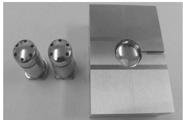
Fig.9 Machined molds (left: cores, right: cavity) [Cutting conditions] Feed rate: 20 \mu\text{m}/\text{rev} , Depth of cut: 5 \mu\text{m} , Cutting speed: less than 0.64 m/min, Cutting fluid: oil mist, [Tool] Material: single crystal diamond, Rake angle: 0 deg, Clearance angle: 10 deg, Nose radius: 1 mm, [Workpiece] Material: die steel (JIS: SUS420J2), Hardness: HRC54, [Vibration conditions] Vibration amplitude: 4 \mu\text{m}_{\text{p-p}} (circular), Frequency: 38 kHz
