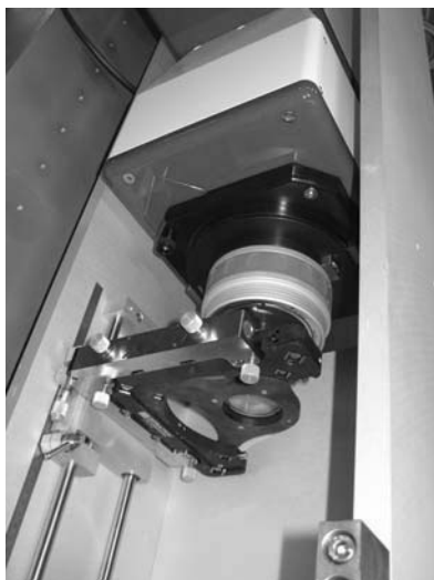
Figure 4. CGH holder, CGH and interferometer optics.
