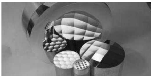
Figure 3. Examples of Complex Surfaces Enabled by Fast Tool Servo Technology.
