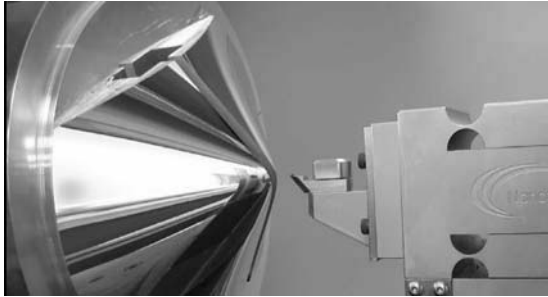
Figure 2. Deterministic Machining of a Highly Aspheric Surface.
