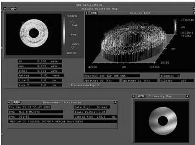
FIGURE 11. *Precessions* achieves 40nm PV ( $\lambda/15$ ) using the morphed error map.
