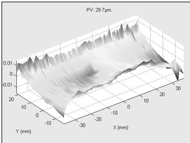
FIGURE 4. Grinding error after compensation: 29.7µm.
