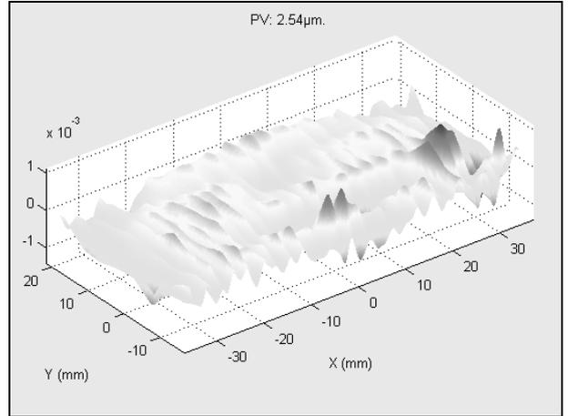
FIGURE 5. Final error after *Precessions* runs: 2.54µm.
