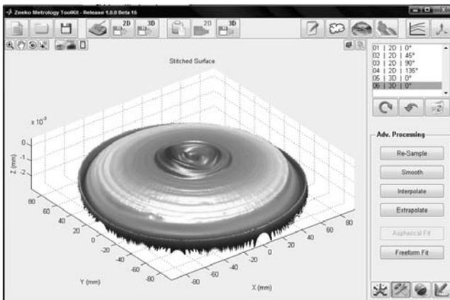
FIGURE 9. Toolkit fuses data sets into a single map.
