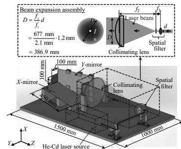
**Fig. 5.** Schematic of the developed optical setup of the compact non-orthogonal two-axis Lloyd's mirror interferometer for fabrication of large area 2D scale gratings.
