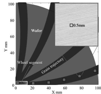
Fig. 2. Cutting path and measurement point.
