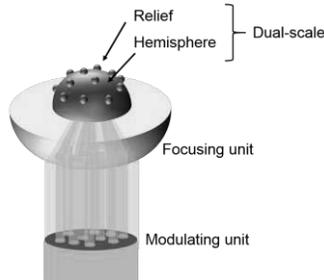
**Fig. 3.** Conceptual figure of the proposed one-shot stereolithography that combines the focusing and modulating units. The modulated light enters the focusing unit and exposes the photocurable resin. A form corresponding to the light-intensity distribution is fabricated.
