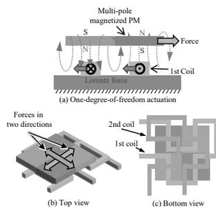
Fig. 1. Principle of two-degree-of-freedom actuation.
