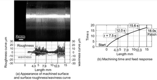
**Fig. 4.** Machined surface and machining time in machining test with respect to increasing spindle rotation speed.
