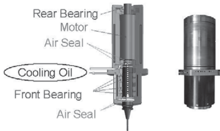
Fig. 2 Highly efficient spindle shaft cooling technology
