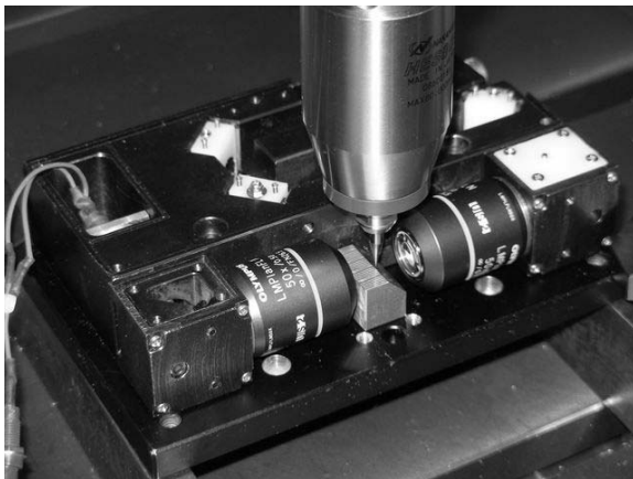
Fig. 3 Outside view of the tip position measurement system
