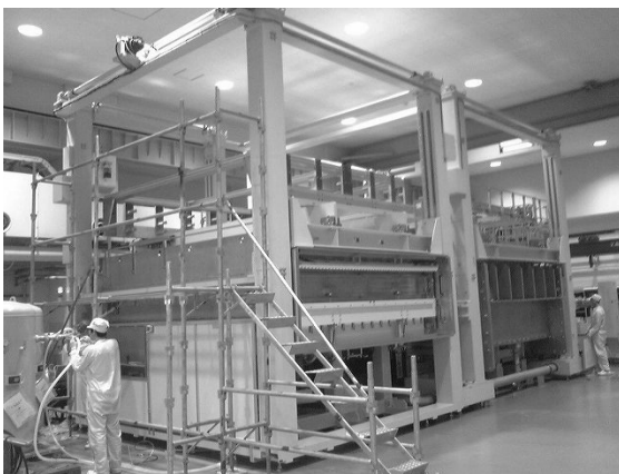
Fig. 3 TFT Array Tester for G10 (Assembling)
